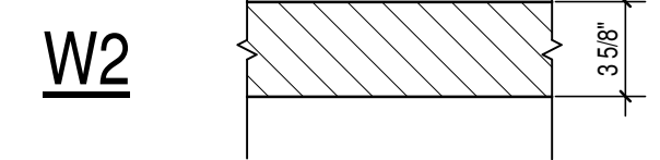
W2 • 3'-5 1/2" CONCRETE MASONRY UNIT
